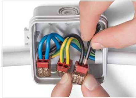
Termination: Insert stripped solid conductor until it hits the backstop.
