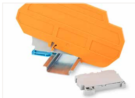
Ex e II/Ex i terminal strip Notice: The movable feet of terminal blocks and separator plates must face the same direction.
