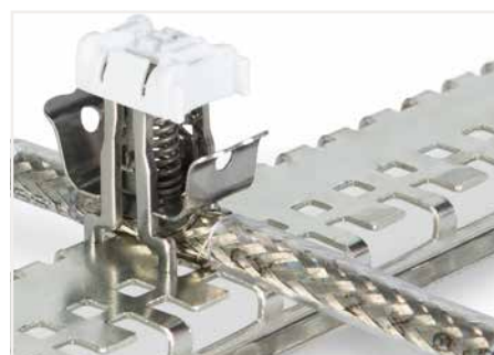
Shield clamping saddle contacts shield conductor and specialty slotted DIN-rail (790-145). Please use the spacer module (790-144) under the rail.
