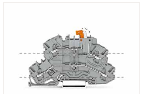
Double-deck disconnect terminal blocks with a pivoting knife disconnect (2002-2671) can be used as through terminal blocks on the lower deck and as disconnect terminal blocks on the upper deck.
