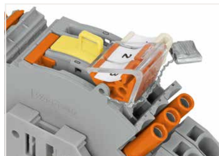
A lock-out seal can be used on the disconnect link in operating position I when combined with an end and separator plate (2007-8893 or 2007-8894).
