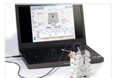
Interface Configuration software, with 750-923 USB Communication Cable
