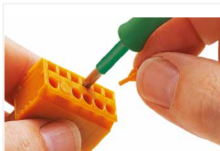
Covering unused clamping units in CAGE CLAMP®-equipped male and female connectors (e.g., when doubling the pin spacing to meet clearance and creepage distance requirements, or when a higher rated voltage is required). Lockout pins are not suitable for panel-mount, angled female connectors.
