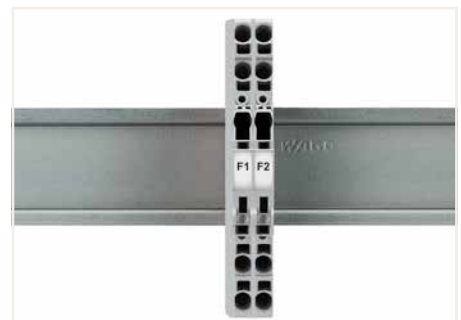
Fuse terminal blocks with a width of 6.2 mm can be assembled adjacently. If there is no adjacent fuse terminal block at the end of the assembly, an end plate must be used.
