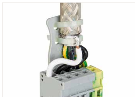
Secure both shield conductor and shield termination (790-350) to the strain relief plate using cable ties.
